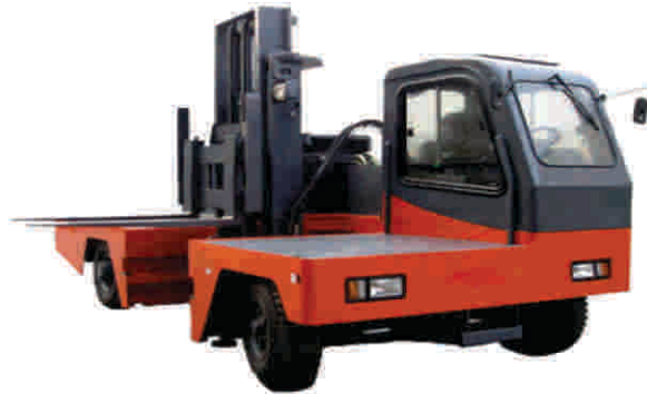
Side Loading Forklift Capacity : 3 - 6 Ton
